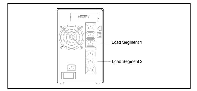
Figure 10. 1000 VA and 1500 VA Load Segments
